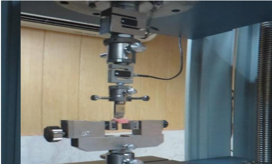
Figure 1. Applying the shear force parallel to the upper base of the brackets at UTM
